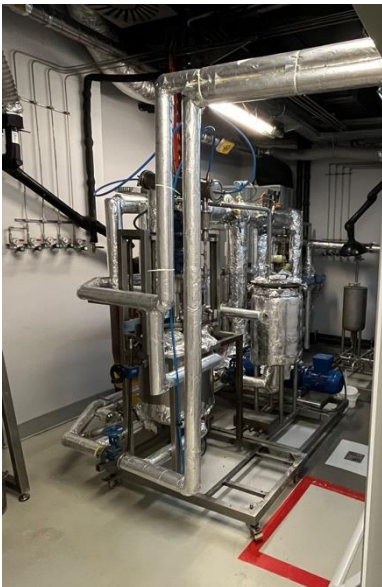
Custom design, tailorable, semi-pilot scale solvent-based recycling system with 40 lt capacity (TRL 6)
