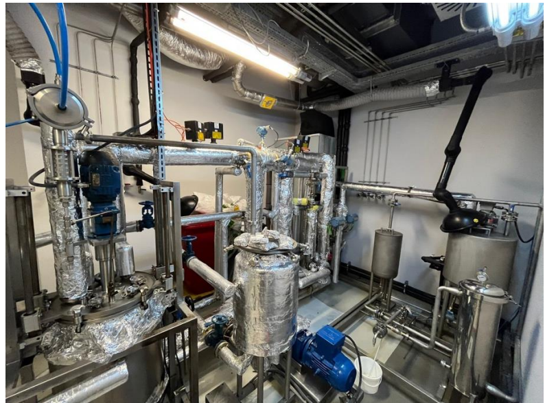
Custom design, tailorable, semi-pilot scale solvent-based recycling system with 40 lt capacity (TRL 6)
